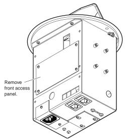
Figure 3-7 — Front access panel removal (HSA 222 models)
